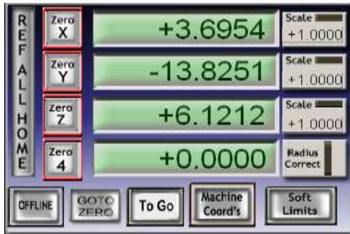
Figure 5. The scale is +1 when using the number of pulse for x-y axis of 3900 and z axis of 4300.
