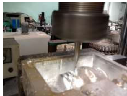
Figure 8. The milling process of a human face.
