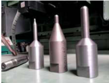
Figure 3. Three forming tools designed specifically for the machine.
