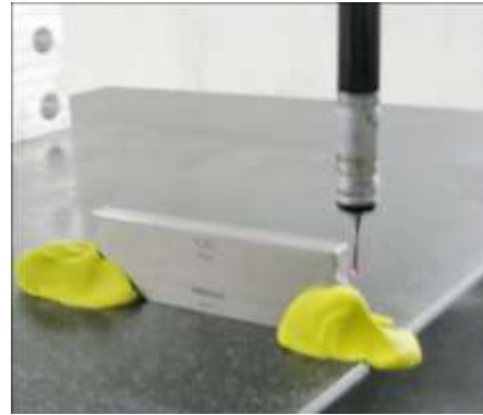
Fig 15. Verification of the calibration method
