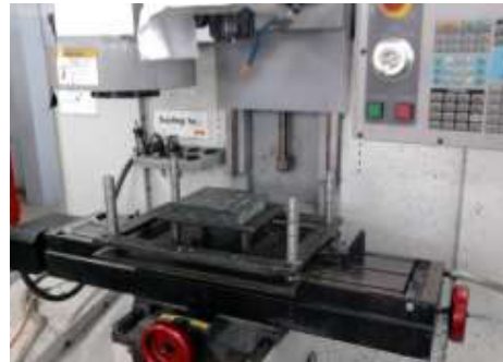
Figure 7. Fixture and work-piece fixed on machine table
