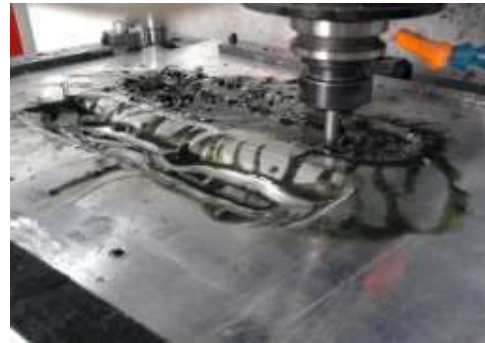
Figure 9. Forming process by TPIF
