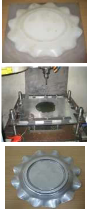
Figure 1. A sample of producing a sheet model by using ISF
