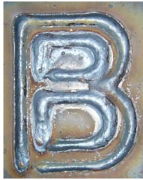
Fig 12. Heat effect on welding path
