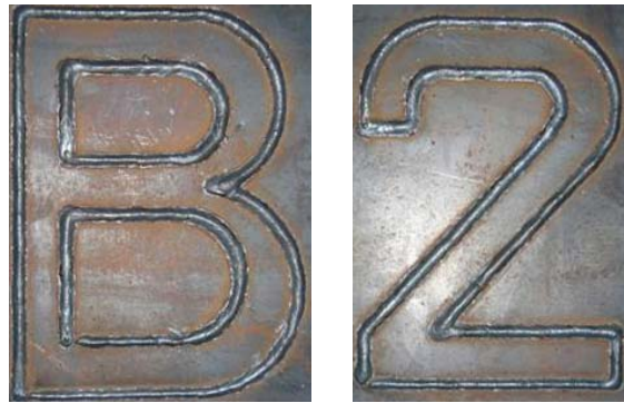
Fig 13. Result of the last welding test
